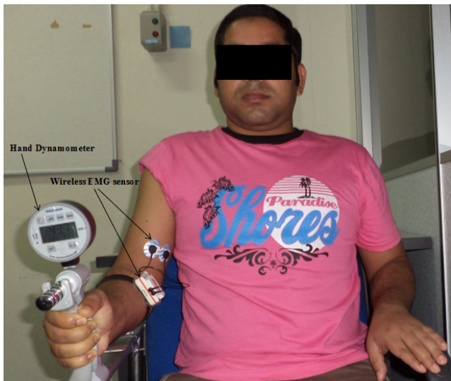
Figure 1: Experimental setup during surface EMG data recording
