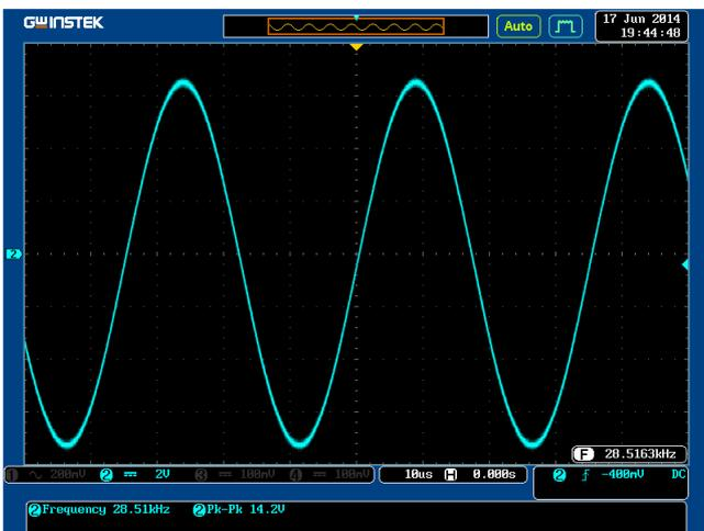
Figure 12. The Output voltage for zero distance case (Volt/div = 10usec , Time/div= 2V)
