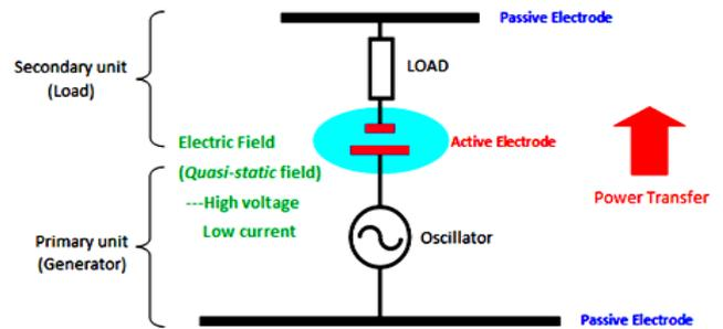
Figure 5. The basic structure of a CPT system [19]
