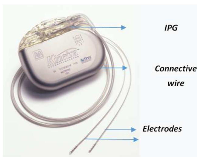
**Figure 1.** Components of a DBS system [12]
