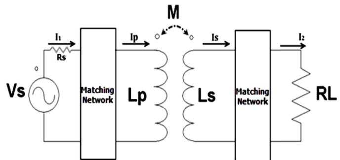
Figure 7. General schematic of a WPT system
