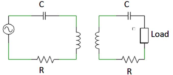
Figure 4. A magnetic resonance circuit
