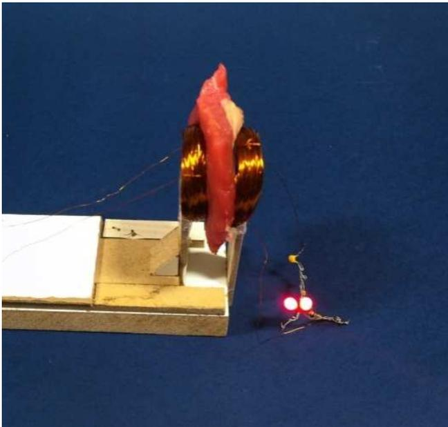
Figure 11. Wireless power transmission through the meat
