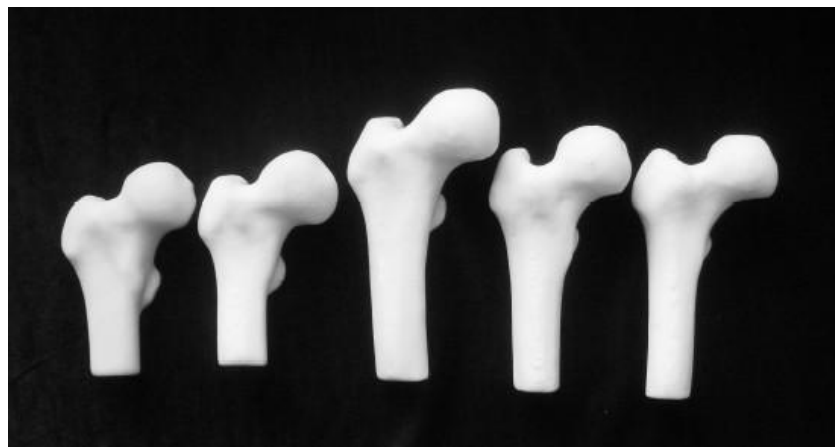
Figure 5. Rapid prototype models of five proximal femurs
